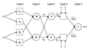
Fig. 1 Architecture of a 2 input ANFIS
